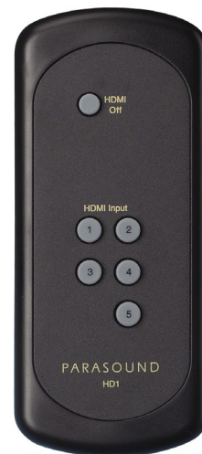
The Zhd remote has discrete IR codes.
