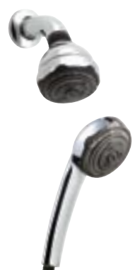
Adlon The Adlon full-sized brass showerhead features 10 dial settings and 8 spray selections. Sprays include drenching full-cone, center jet, turbo massage, pulse massage, slow pulse massage and two combination variations. It also features a watersaving trickle valve at each end of the dial. Self Clean prevents clogging and corrosion. Solid brass construction.
